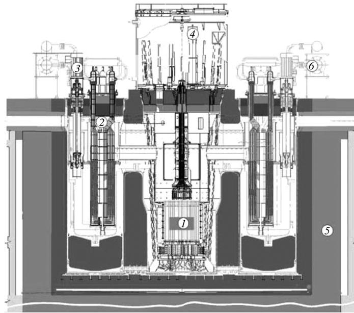
Fig. 3. BREST-OD-300 reactor: 1) core; 2) steam generator; 3) pump; 4) reloading machine; 5) shaft; 6) cooldown system.
