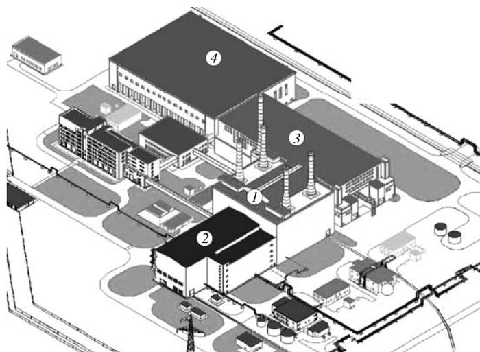
Fig. 2. Nuclear power complex with a BREST-OD-300 reactor: 1) reactor; 2) turbines; 3) complex for storing and reprocessing radioactive wastes; 4) complex for the on-site nuclear fuel cycle.
