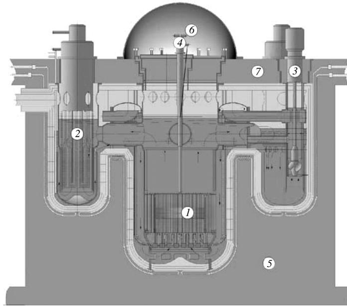
Fig. 1. BREST-1200: 1) core; 2) steam generator; 3) pump; 4) reloading machine; 5) reactor shaft; 6) sealing cap; 7) top plate of cover.
