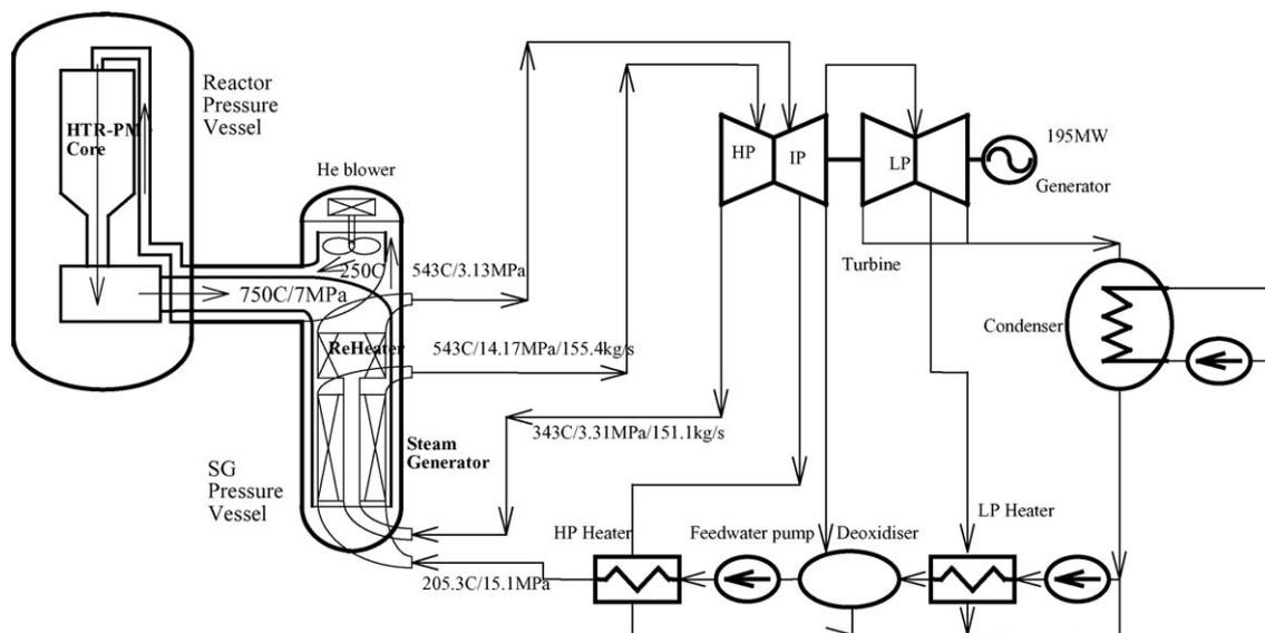
Fig. 2. Flow diagram of the HTR-PM steam turbine cycle.
