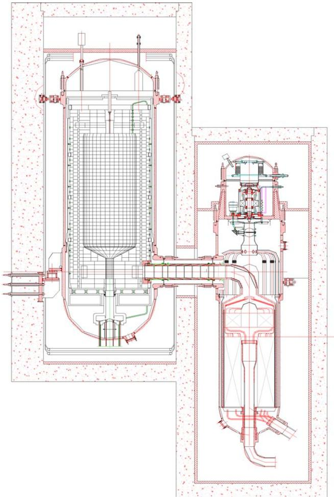
Fig. 1. Primary system of the HTR-PM.
